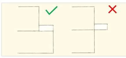
**Figure 68.3.1:** permitted vs. prohibited forms of balconies for residential units above non-residential uses as per 68.3(1)(a) of this section.
