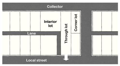
Figure 60.3.1: an illustrative guide to lot types as per 60.3.1(1) of this section.
