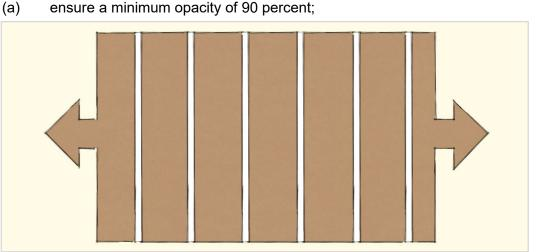
Figure 77.2.1: an example of screening with approximately 90 percent opacity.
