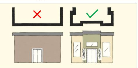
Figure 60.2.1: an example of façade articulation as per 60.2.2(1) of this section.
